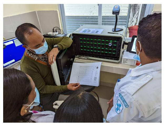
Caption: The laboratory director from Maubisse referral hospital explaining the process for using and maintaining the new Bactec machine, which is used for blood culture testing.
